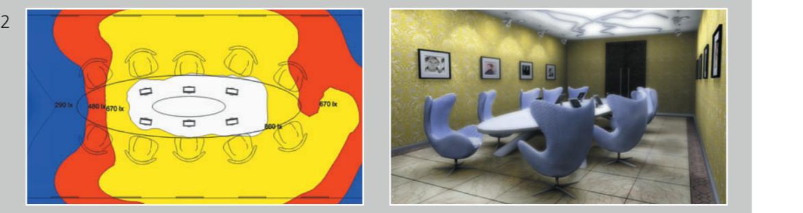
1 PYTHA RadioLab utilizes the radiosity method of lighting calculation taking into consideration the aspect of 'indirect light' and surface properties. This results in an extremely realistic lighting representation of an interior. Virtual photometry can be determined during the planning period.
